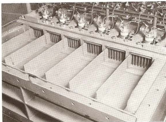
Part of the thyristor frame showing the arrangement of the cooling fins
